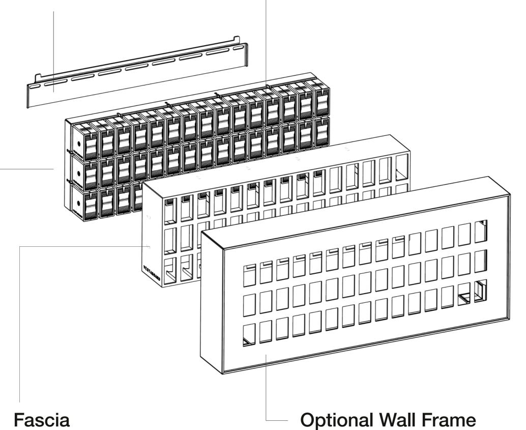
The fascia covers and protects the Bits while keeping them securely in place. It can be removed to access individual Bits for replacement or maintenance, but ensure it is attached to the backplane if mounting to the wall plate.
